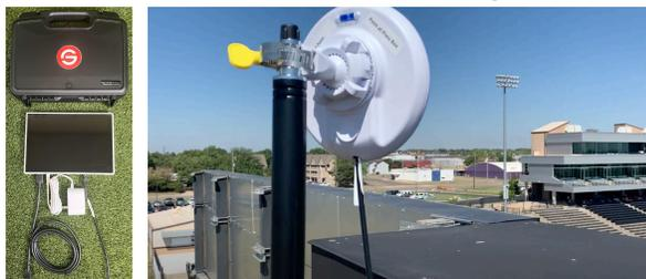
\*camera station & end zone antennas should have a clear line of sight to the press box, no obstructions
