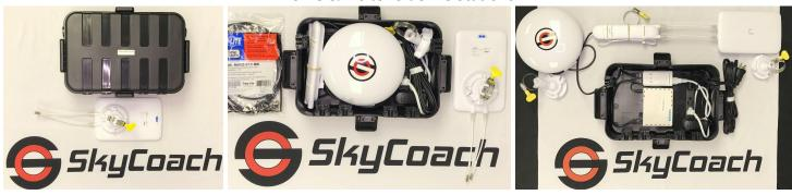
\*each sideline station has a power box with a stickered antenna and a "wifi" antenna
