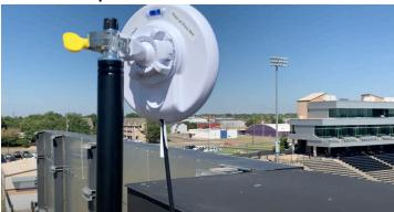
\*be sure the antenna has a clear line of sight to the press box antenna
