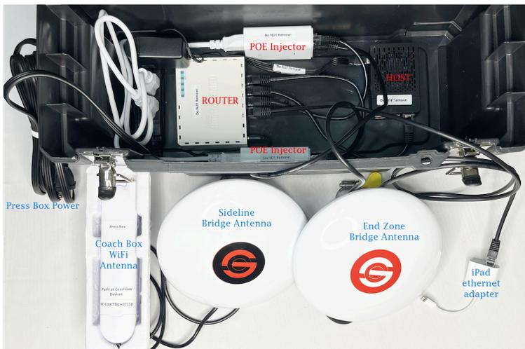
\*the network diagram on the next page details where the cables are plugged
