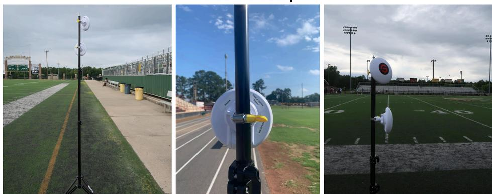
\*station should be placed at the 35 yd line, farthest from the bleachers with a clear line of sight to the press box antenna
