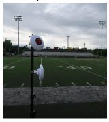
\*station should be placed at 35 yd line, farthest from bleachers, with a clear & straight line of sight to press box antenna
