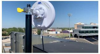
\*be sure the antenna has a clear and straight line of sight to the press box antenna
